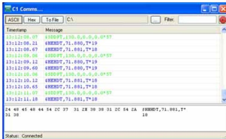
The data received on the port is displayed green and the data sent on the port displayed blue as shown in **Figure 9-11**. The communications can be saved to a file by selecting a location and clicking the **To File** button. The communications can be filtered by entering Filter text. Any communication containing the filter text is displayed red as shown in **Figure 9-12**.
