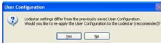
5. Refer to **Figure 6-18**. If the Lodestar is not connected the software will prevent the user accessing any windows to retrieve or configure Lodestar settings.
