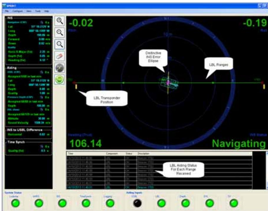
If any LBL ranges are rejected, the LBL aiding ‘traffic light’ will change to amber/orange and the beacon address and reason for rejection will be displayed. Examples showing reasons of LBL rejection are shown in Figure 9-7.
