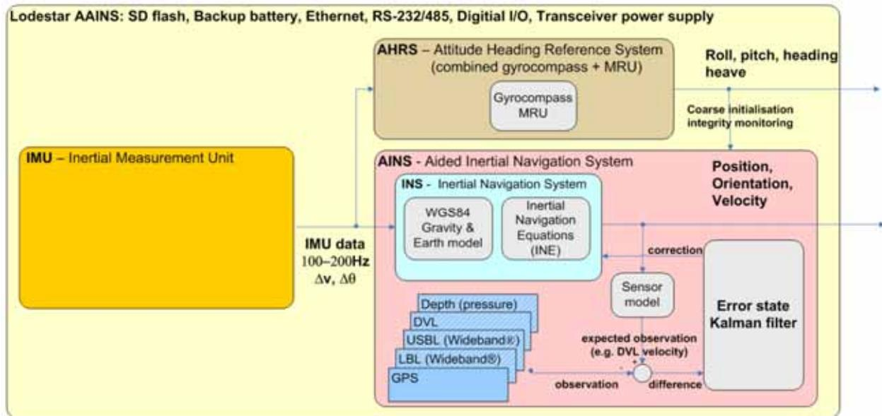
The INS aiding options available in SPRINT are listed in **Table 3-1**. Only certain position aiding inputs, such as USBL can be used to initialise Inertial Navigation and that these aiding inputs must be UTC time synchronised.
