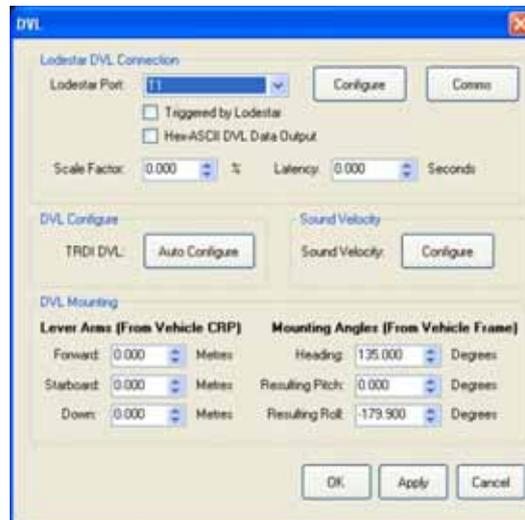
2. Refer to **Figure 6-26**. Select the **Lodestar DVL Connection** port from the drop down menu, click **Apply** to set the port before continuing.
