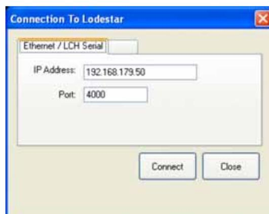
3. Refer to **Figure 6-15**. Click **Connect**. If this is the first time the system has been run and connected to the Lodestar it will then configure communications routing and 'pipes'. It may take several minutes for this process to complete; a progress indicator will be displayed.
