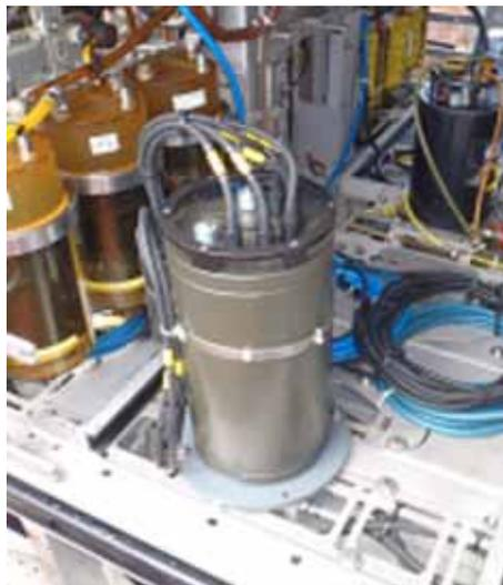
In this arrangement the X-axis indicator on the top of the Lodestar is aligned with the forward direction of the vehicle reference frame and the Y-axis indicator is aligned with the starboard direction of the vehicle reference frame (refer to **Figure 5-3**).
