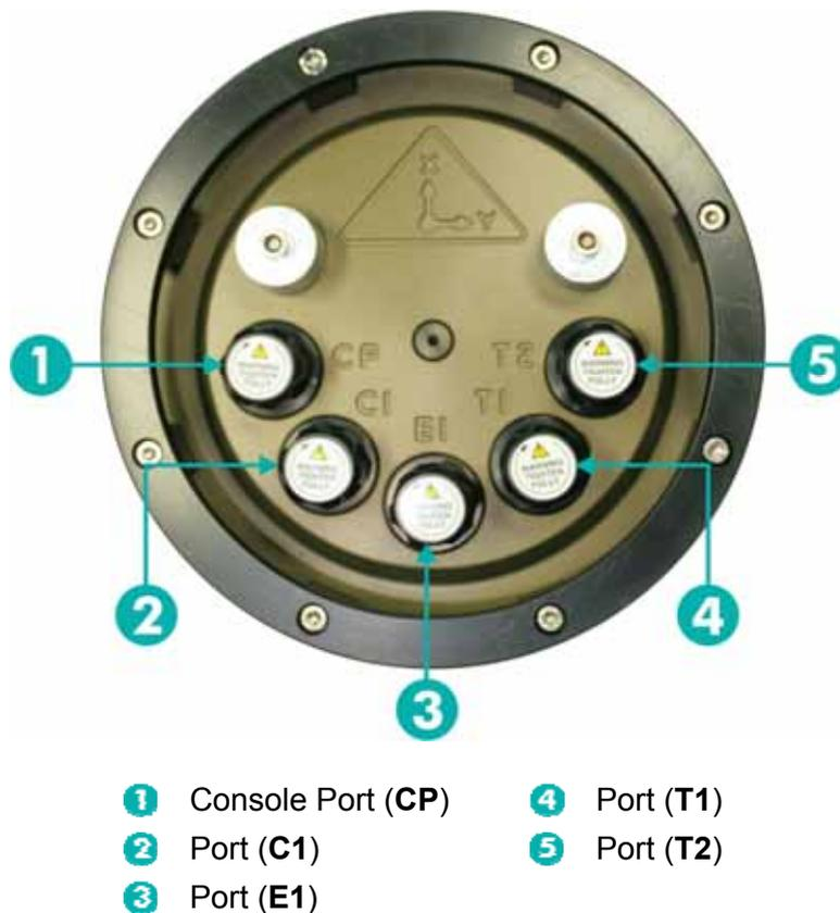
2. If a Pressure Depth Sensor is to be connected to the Lodestar, connect to Port **C1** 2.
