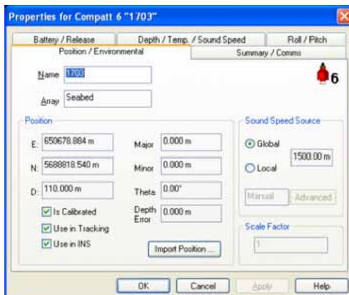
27. The ROV can now be tracked using INS with LBL aiding. Click the green **Go** button to start the tracking wizard.
